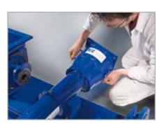
8. Remove the stator
