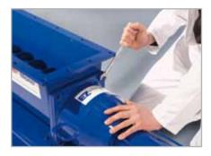
2. The feed chamber is pulled back to allow full access to the pin joint area for removal of any blockages or compressed cake
