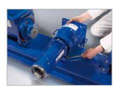
6. Unscrew the rotor from the stator
