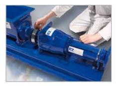
5. Turn the feed chamber and rotor and stator into position and secure
